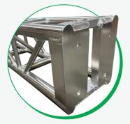
Guardian's unique connection plate extrusion provides support and protection for the ends of the chords reducing the risk of tube damage. The design also provides up to 10% more truss load capacity compared to conventional TOMCAT Light Duty 12" x 12" truss utilizing standard end plates.
